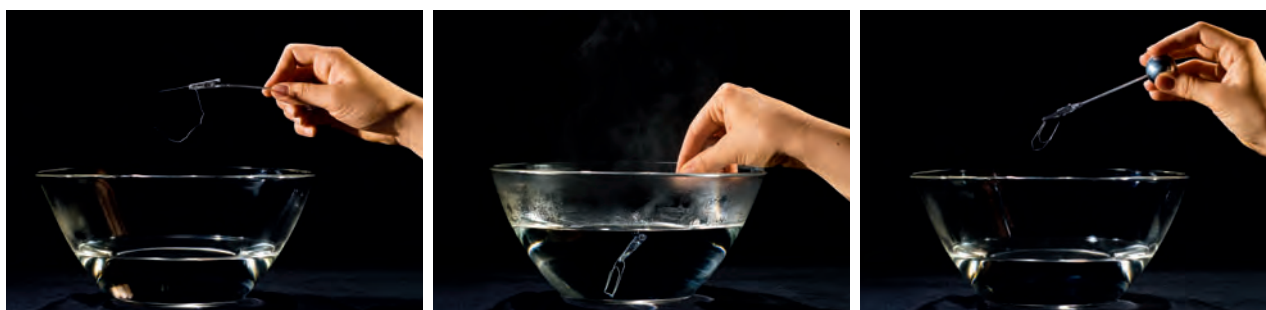
Live wire: Immersion in warm water enables the bent paper clips to return to their fully functional shape. The extent to which they can be bent while cold is determined by the number of possible microstructures.
