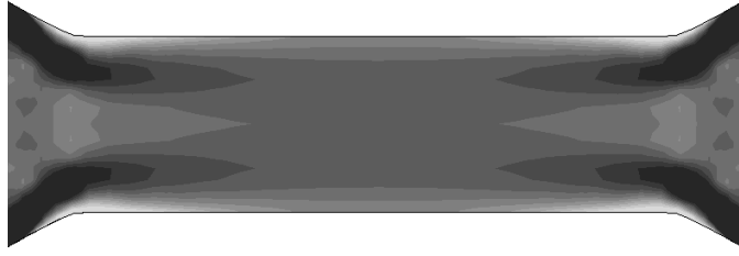
FIGURE 5. Density plot of the von Mises stress at stretch s = 1.38 . For greater clarity, the full sample is displayed here (computations have been performed on one quarter only).
