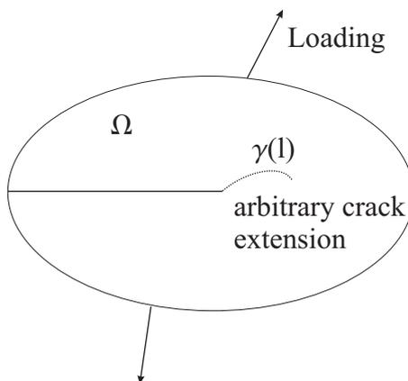
FIGURE 3. Energy released by an arbitrary virtual extension.
