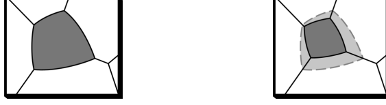
Figure 3. Hypothetical annealing process. Left : unit volume containing a shrinking crystallite (gray). Right : after a unit time interval, the gray crystallite has lost the mass indicated by the dashed region, viz. \varrho^* \Gamma^* < 0 . Accordingly, the dislocation loss is given by \rho_{\text{D}}^* \Gamma^* .
