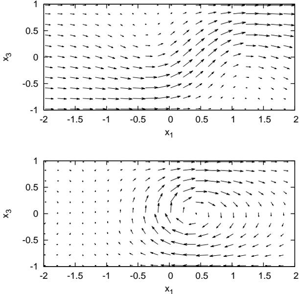
Fig. 1. Stray-field free domain walls: Asymmetric Néel (top) and asymmetric Bloch (bottom) wall.
