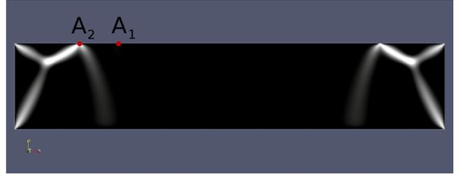
Fig. 6. Domain walls as simulated by the diffuse interface model. A doublet is pinned via the boundary conditions at the point  $A_2$  (and symmetric on the other side).  $A_1 \in \partial\{|\mathbf{m}^*| = 1\} \cap \partial\omega$  indicates one of the transition points at the boundary from the non-saturated to the penetrated region.
