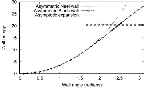
Fig. 4. The energy of asymmetric domain walls,  $L = 10$ ,  $500 \times 50$  cells in the grid.
