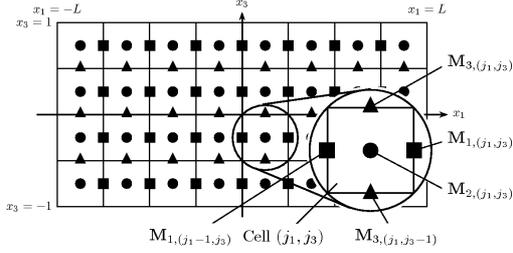
Fig. 3. The staggered grid used to discretize  $E_{\text{asym}}$ .
