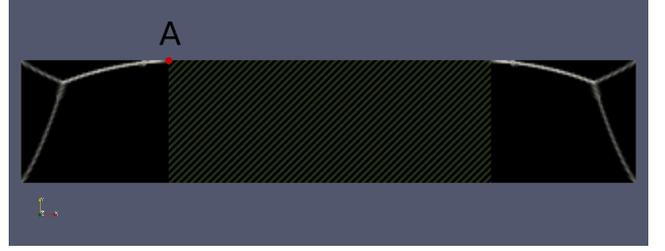
Fig. 5. Domain walls as simulated by the viscosity solution selection criterion for a penetrated sample.  $A \in \partial\{|\mathbf{m}^*| = 1\} \cap \partial\omega$  indicates one of the transition points at the boundary from the non-saturated (plain black) to the penetrated region (striped pattern).
