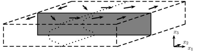
Fig. 2. The cross section of a ferromagnetic sample transversal to a domain wall. With indicated asymmetric Bloch wall.
