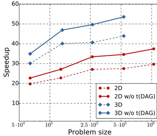
Figure 15: Scaling of  $\mathcal{H}$ -LU factorization speedup for 60 cores and an increasing problem size for nested dissection in  $\mathbb{R}^2$  and  $\mathbb{R}^3$ .
