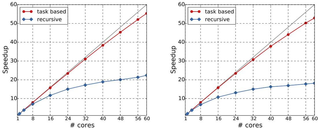
Figure 12: Speedup of task-based and recursive  $\mathcal{H}$ -LU factorization for Helmholtz kernel on a sphere (left) and cylinder (right) grid.
