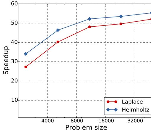
Figure 13: Scaling of  $\mathcal{H}$ -LU factorization speedup for 60 cores and an increasing problem size for Laplace and Helmholtz kernel.
