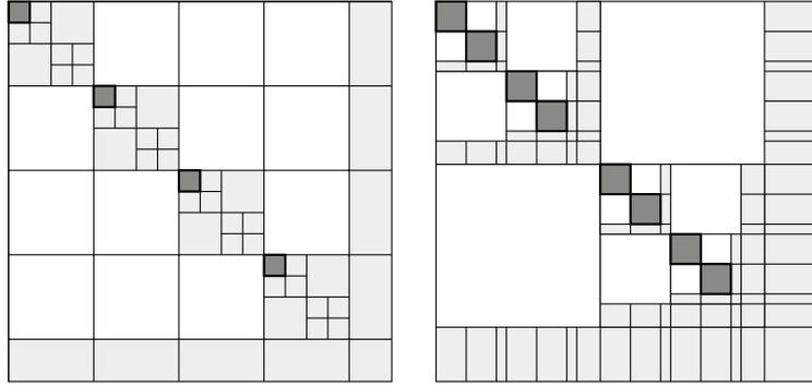
Figure 8: Matrix structure for the domain decomposition case (left) and nested dissection case (right).
