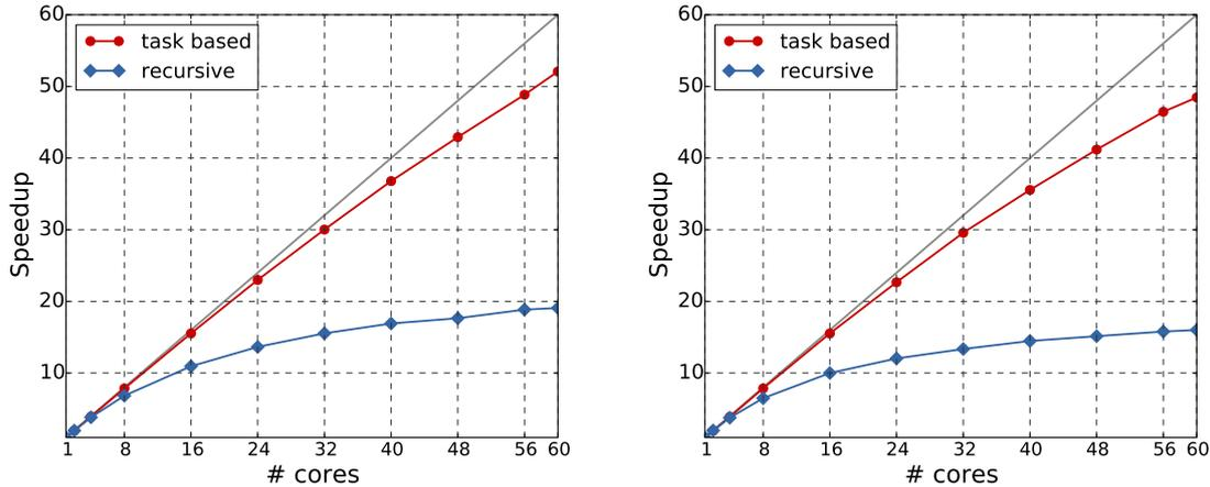
Figure 11: Speedup of task-based and recursive  $\mathcal{H}$ -LU factorization for Laplace kernel on a sphere (left) and cylinder (right) grid.
