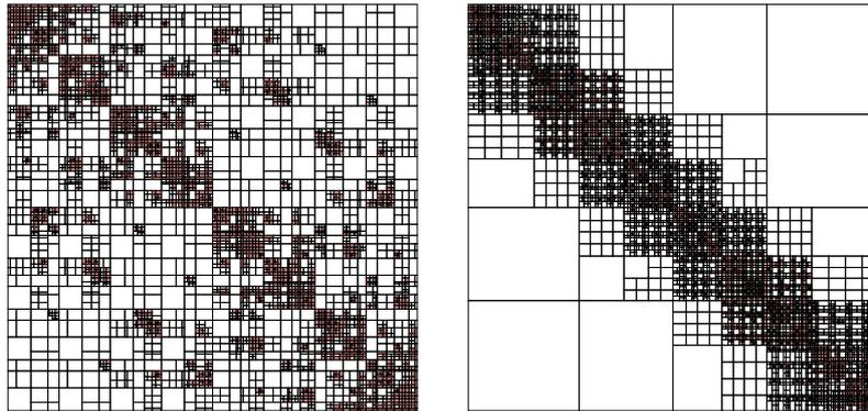
Figure 10: Block partitioning for the sphere (left) and cylinder (right) grid.
