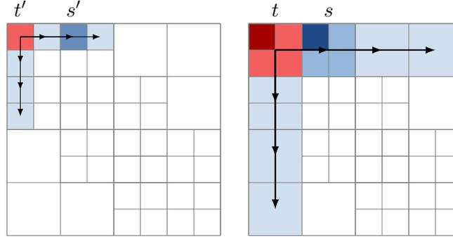
Figure 4: Example of multiple solves per matrix block due to double recursion.
