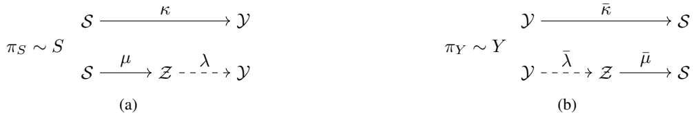
Fig. 1: (a) Simulation of the channel \kappa by a randomization at the output of \mu . \kappa and \mu share a common input alphabet \mathcal{S} . (b) Simulation of the channel \bar{\kappa} by a randomization at the input of \bar{\mu} . \bar{\kappa} and \bar{\mu} share a common output alphabet \mathcal{S} .
